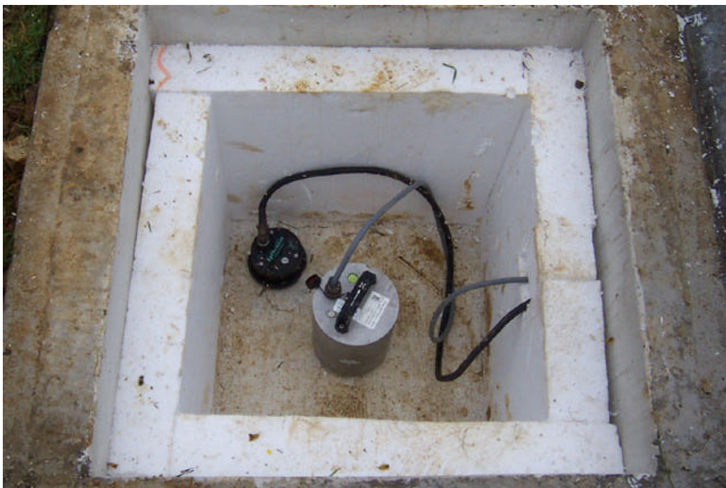
Figure 3. A view of a NZNSN vault with a Guralp CMG-3ESP broadband seismometer and Kinematics Episensor installed.
