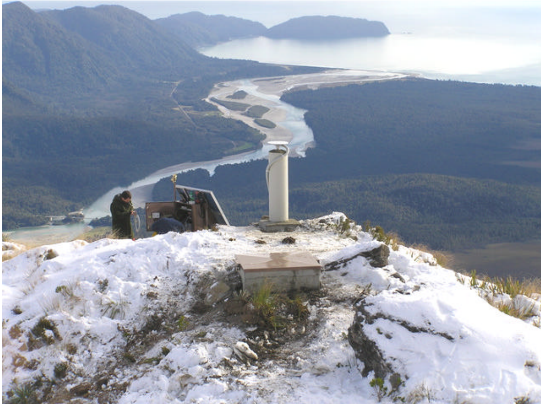
Figure 5. The remote NZNSN site above Jackson's Bay in South Westland. This is a joint CGPS site. The vault is in foreground, the CGPS pillar and equipment cabinet in background with Jackson's Bay in the far background. The data is radioed via Ethernet bridge to Neill's Beach where a VSAT installation transmits the data to the GeoNet data centre.
