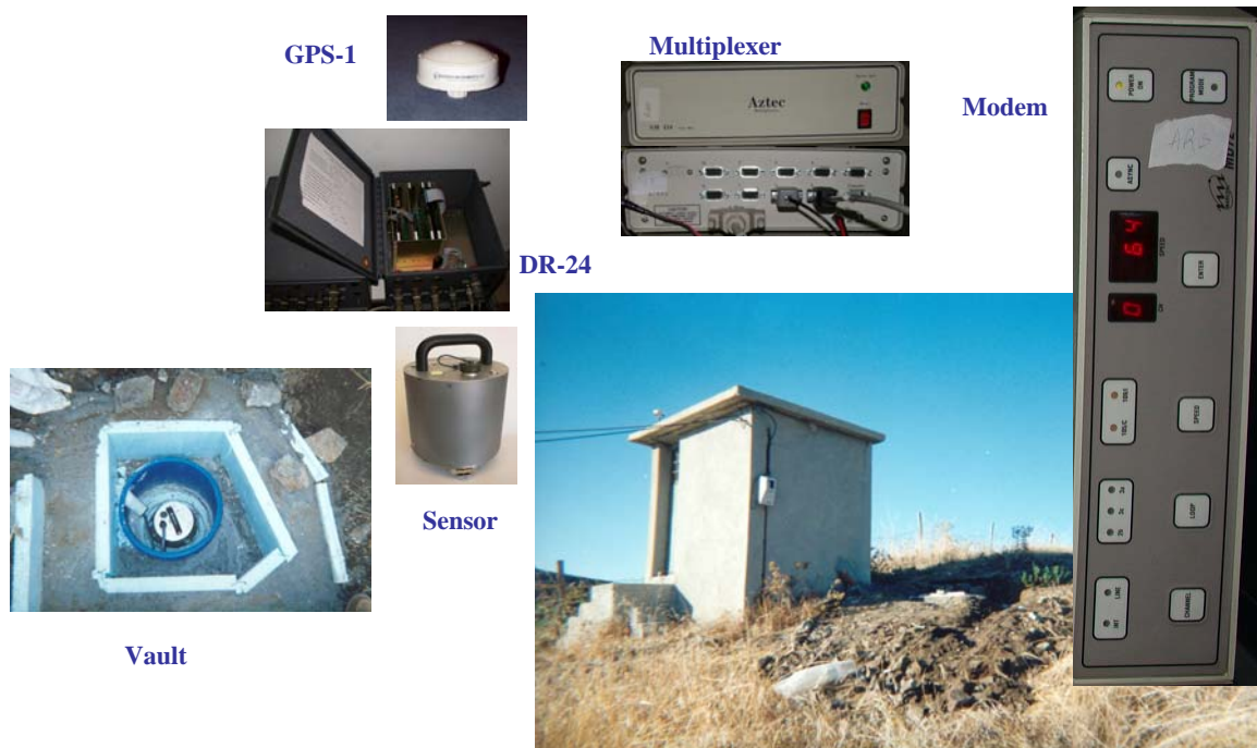
Figure 4. A typical HL outstation. In the present case LIA site.
